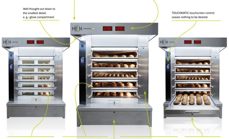
Steam-tight oven doors made of stainless steel. Fitted with Sekurit glass on request (at no extra charge).
