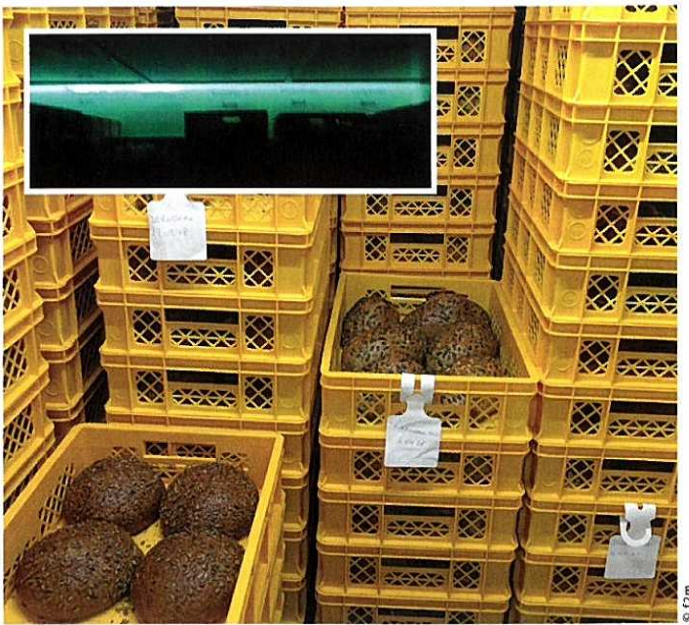
++ Various bread types, sorted and with date labels, are stored in crates in the Flexbaker. Photo top: When the Flexbaker is closed, the UV lamp along which air circulates can be seen
