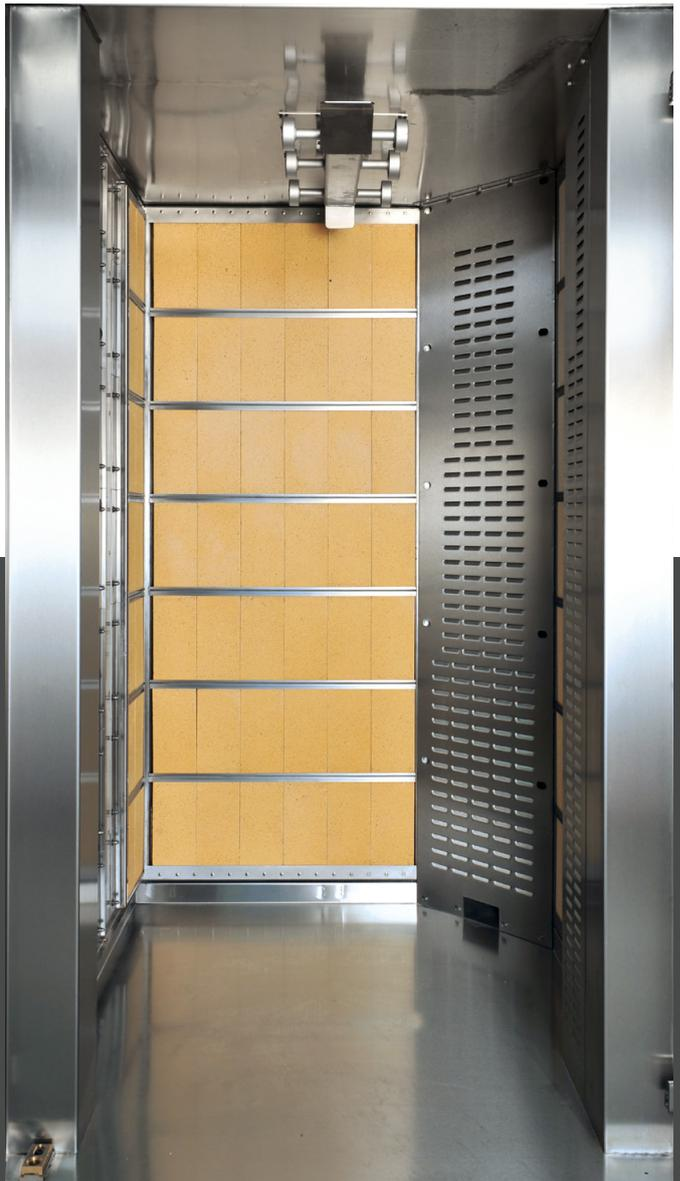
*Baking chamber with head suspension*
